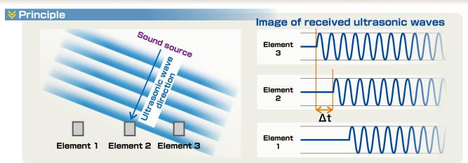
Ultrasonic waves are caught by array sensor consisted of elements, and there are time distance ( $\Delta$ t) in waveforms received by the elements. It occurs from angle from sound source direction. MK-750 finds the direction of the sound source = the leak point.
